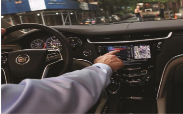
Cadillac's CUE touch-less control system uses infrared sensors to interpret hand gestures.
